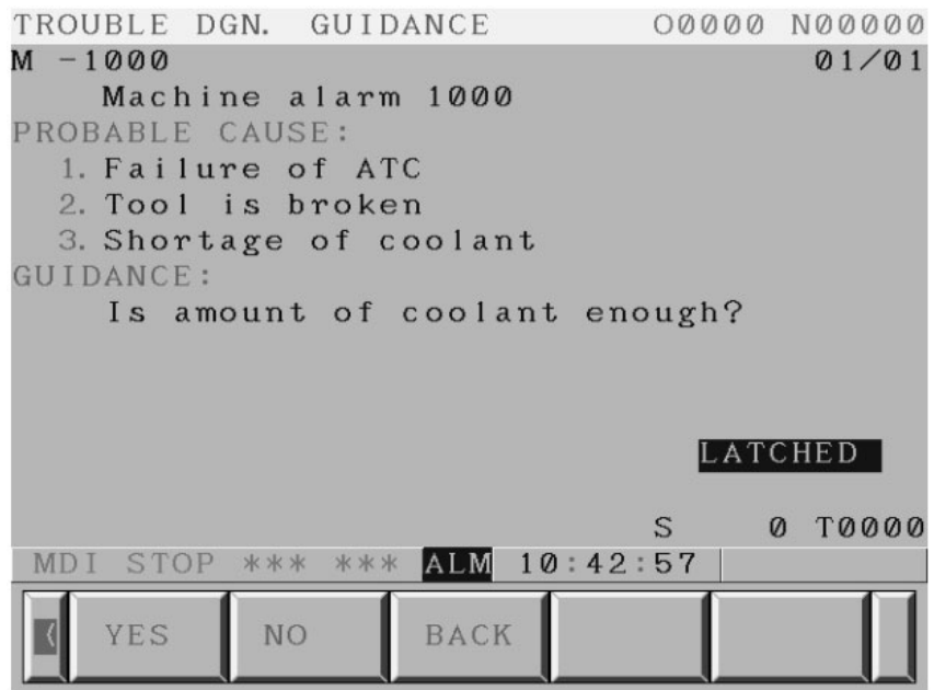
Example of a trouble diagnosis guidance screen
